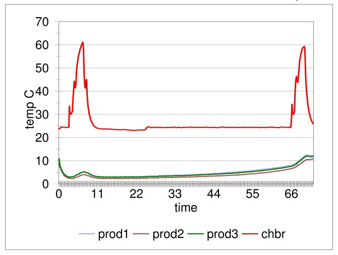
Box: 12" x 12" x 13" with 1.5" Blue Control Temp Test Duration: 72 hours Product: 3 - Empty 100 ML Bottles
