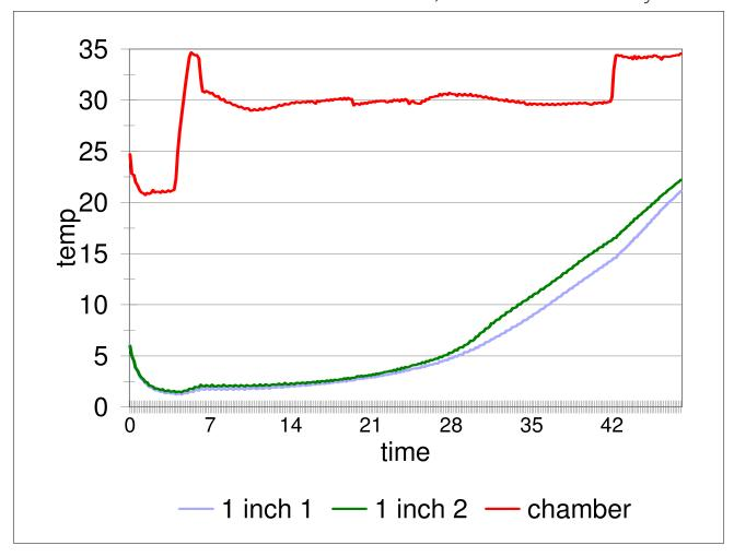
Box: 12" x 12" x 12" with 1" Classic Control Temp Test Duration: 48 hours Product: 5 - .5ml syringes in 5 packs. Total 25 syringes in corrugated load box. Coolant: 6 -16-ounce Gel Paks frozen at -20°C
